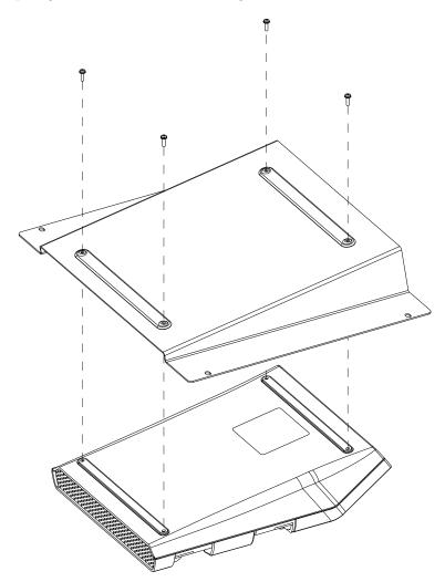
3. Offer up the DL Series mixer to the rack and secure it in place with four rack screws (not supplied). Be sure to use the PadLock included with your mixer to ensure that the iPad stays safe and secure during transport with the mixer. Also, remember to leave enough room at the top of the rack to attach the DC power cord and any other connections needed.
