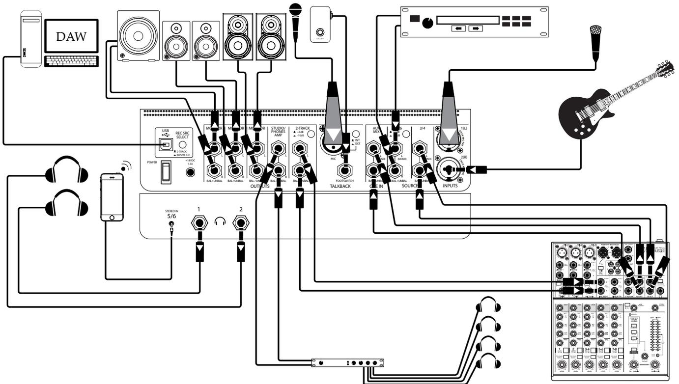
The Big Knob Studio+ is similar to the Big Knob Studio, but with a few more bells and whistles. No time to waste, let's get started! In this example, a microphone is connected to XLR input 1 (L) and a guitar to 1/4" input 2 (R). The Source Input 3/4 jacks are connected to an external mixer's Control Room (CR) output jacks, playing whatever sounds / sources are fed into the mixer. Likewise, the Cue In (Aux Mix) jacks are connected to the same mixer's Alt 3/4 output jacks.
