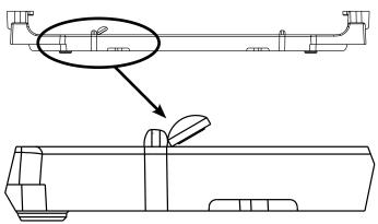
4. Keeping the rail strip butted up next to the tray insert's rail, continue to apply pressure while pushing the rail strip down against the tray insert until the adhesive sticks.
