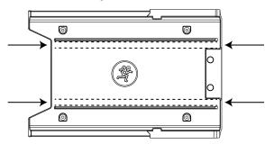
2. Doing your best to not touch any part of the adhesive, remove the adhesive backing paper of one of the iPad Air 2 rail strips.
