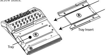
9. Place the screws back into the DL mixer from where they were removed. Screw them into place, but do not overtighten. If the iPad fit is too tight, loosen all four screws, then tighten the ones closest to the connector first.
