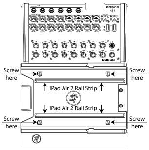
10. To use the PadLock<sup>™</sup>, you will need to install the two nylon washers (included in this kit). Align them flat against the threads of each PadLock screw<sup>™</sup>, put the driver into the screw head and slowly turn the screw to thread the washer over the screw threads. Apply moderate pressure against the washer while turning the screw so the washer threads. Stop when the washers clear the screw threads.
