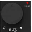
This knob is used to adjust the channel 1 volume - microphone and headset - to the headphones and mix minus.
