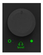
This knob is used to adjust the volume at the 1/4" headphones and 1/8" headset outputs from  $\infty$  (off) to maximum gain (max). Make sure that this knob is fully off before selecting or adding a new source.
