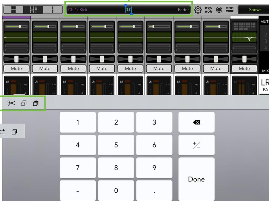
Also, if you want to type in an exact value for a parameter, touch the channel's parameter you would like to update so it appears in the current parameter display. Next, tap the current parameter display; a numeric keypad appears. Simply type in the exact value you would like for that channel's parameter followed by tapping the "Done" button.
