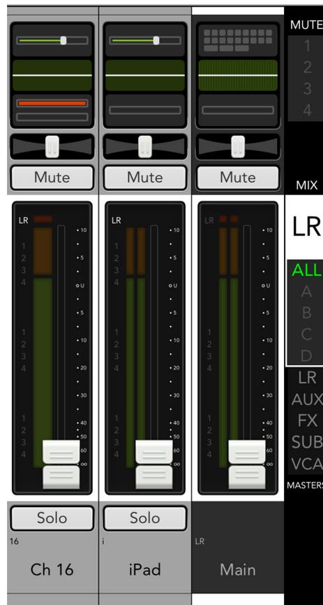
**No High-Pass Filter** — There is no high-pass filter on the iPad channel, so it will be absent in the EQ view for this channel.
