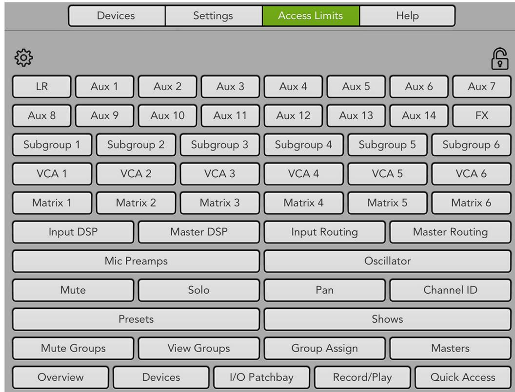
With no access limits buttons pressed, the iPad can access all controls. With one or more buttons pressed, the corresponding control will be hidden and cannot be accessed or changed from that iPad. The function of the limiting buttons is described below.
