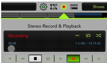
If access to the microphone had previously been set up, then recording will begin immediately. The record button illuminates green when engaged (as see to the left) and is gray when disengaged. Additionally, the international symbol for a recording in progress is a red dot. The record button on the navigation bar will turn from green to red to indicate recording. A third and final indicator is the "Recording" – in red text, no less! – that lies within the Stereo Record & Playback window.
