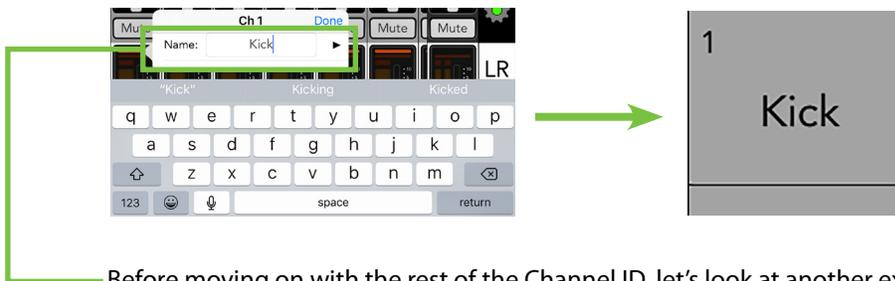
Before moving on with the rest of the Channel ID, let’s look at another exciting feature regarding channel naming. On the left and right side of *Name:* are “previous” and “next” arrows<sup>5</sup>. This makes it easier to edit the names of multiple channels in a row without having to re-tap each channel’s ID button just to name it.
