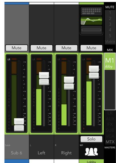
All matrix outputs may be viewed simultaneously by touching the masters selector located at the bottom right of Master Fader.
