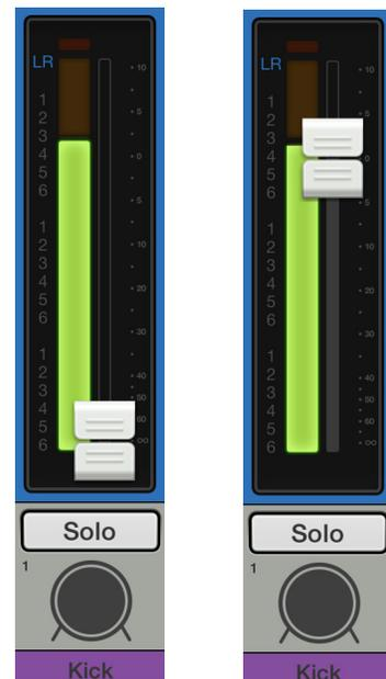
**(6) Less Than Zero** — The gain should be completely off and channel fader all the way down for each channel not in use.
