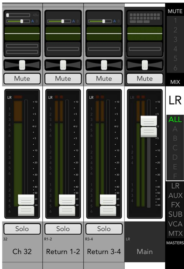
**48V / Gain** — By default, 48V and gain on the return channels is absent from the input routing view for these two channels. However, the source and trim will still be displayed and input routing may still be accessed in order to update channel and aux send assignments.
