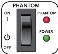
**(1) Phantom Power** — Every DL1608 and DL806 has a global phantom power switch (located on the rear panel of the mixer) that affects all mic channels' XLR jacks simultaneously. If any connected mics require an extra 48V of power, engage the phantom power switch. The accompanying phantom power LED will illuminate red, indicating that phantom power has been engaged.
