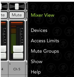
Tap the the gear icon to open up the tools view. Notice that it has a nearly identical layout to that of the tools section of Master Fader for iPad. Master Fader for iPhone is divided into five sections: devices, access limits, mute groups, show and help.
