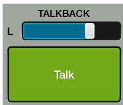
**Talkback** — The DL32R has a talkback level (L) and button. Channel 32 is the default for the talkback input. The talkback level slider controls the level of the talkback mic with the gain ranging from  $-\infty$  to +10 dB. Talkback may be routed to the main L/R, any subgroup, aux send and/or matrix. Refer to the I/O patch on pages 184-196 for more information.
