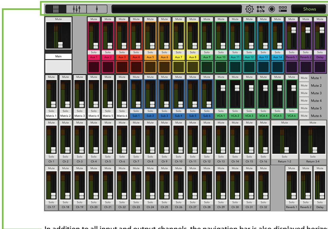
In addition to all input and output channels, the navigation bar is also displayed horizontally at the top of the screen. In fact, the navigation bar never leaves; it is at the top of every view.
