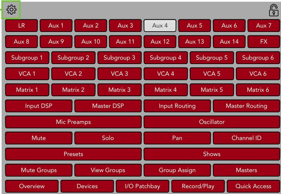
Upon return to the mixer view, you can see that only Aux 4 is accessible. Notice on the far right that Aux 4 is the only available output and that the output selector can't even be opened. Other than that, every other control has been hidden. This makes the faders and meters larger and removes unnecessary information from the interface.
