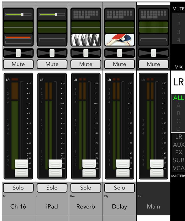
**No Digital Trim** — There is no digital trim on FX channels, so it will be absent from the input routing view for these two channels. However, input routing may still be accessed in order to update channel and aux send assignments.
