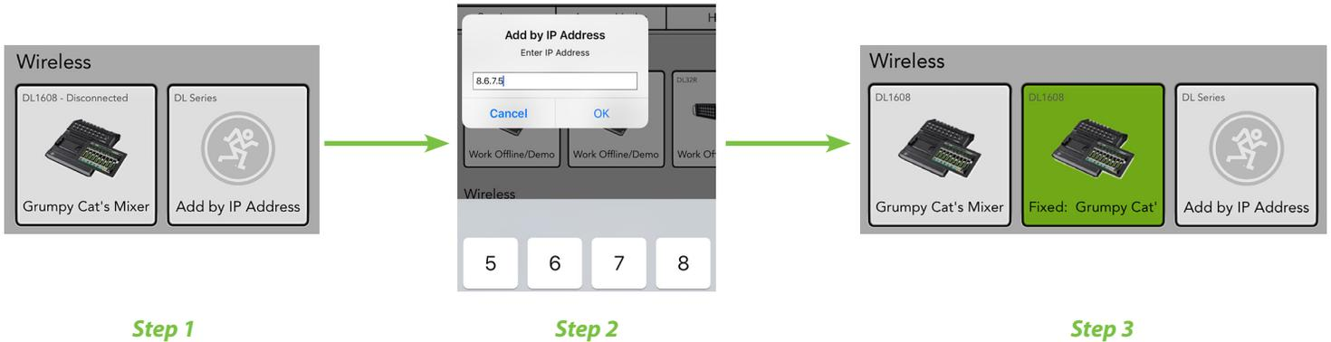
**NOTE** This device will always be shown even if the device is not currently on the wireless network. If the mixer is not present when selected, it will shown Disconnected as described earlier...
