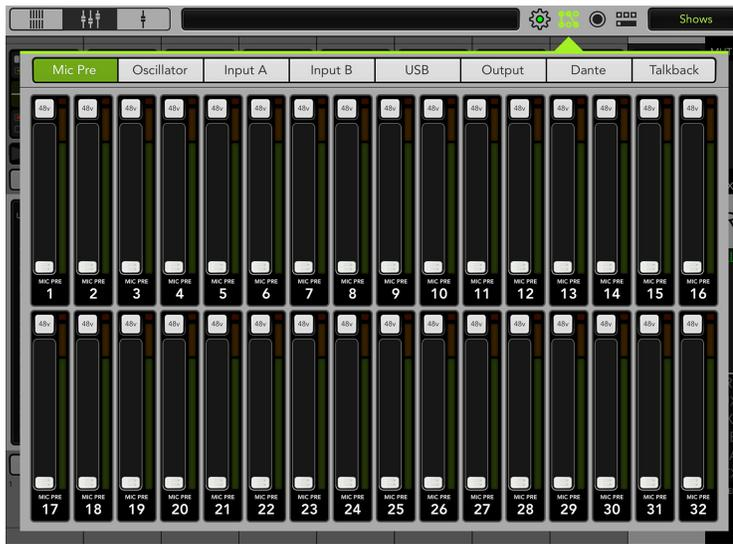
Captain Obvious says, “The mic pre tab is where you adjust the mic pre gains and 48V phantom power in one convenient location.” Don’t you just love it when something is named for what it does?! Not only are mic pre settings made here, but meter levels are also displayed for fast, easy adjustment. Because all mic pres are present in one view, this is extremely useful when the DL32R is used as a digital snake with another console via Dante.
