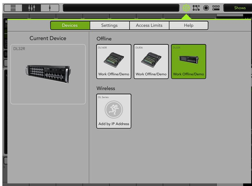
**Wired I [DL1608 / DL806]** — Slide the iPad into the mixer. You will see that the wired device changes to display the name of the DL Series mixer and it is automatically selected. When this happens, a pop-up appears indicating that the console is connecting and synchronizing the current show and then the current state.
