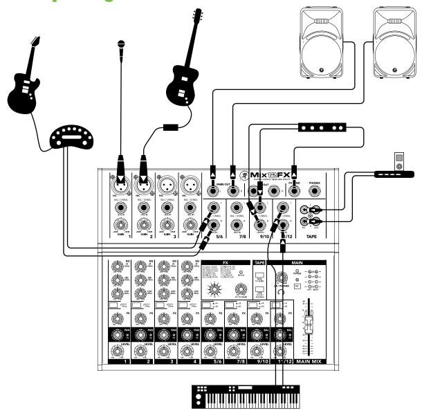
Mix Series mixers are powerful tools that offer a lot of features, but are still easy to set up and use. Let's take a look at an example of using a Mix12FX in a live PA environment.
