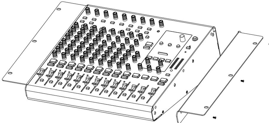
4. Offer up the mixer to the rack and secure it in place with four rack screws (not supplied). Remember to leave enough room at the top to attach the AC power cord and any other connections needed.
