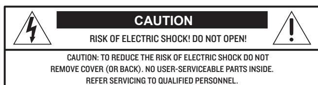
The lightning flash with arrowhead symbol within an equilateral triangle is intended to alert the user to the presence of uninsulated "dangerous voltage" within the product's enclosure, that may be of significant magnitude to constitute a risk of electric shock to persons.
