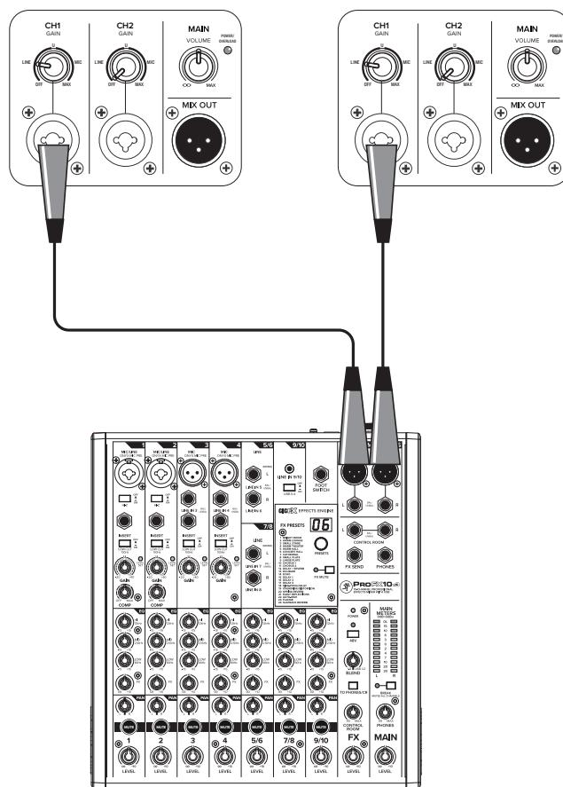
**Using a microphone and daisy-chaining**
