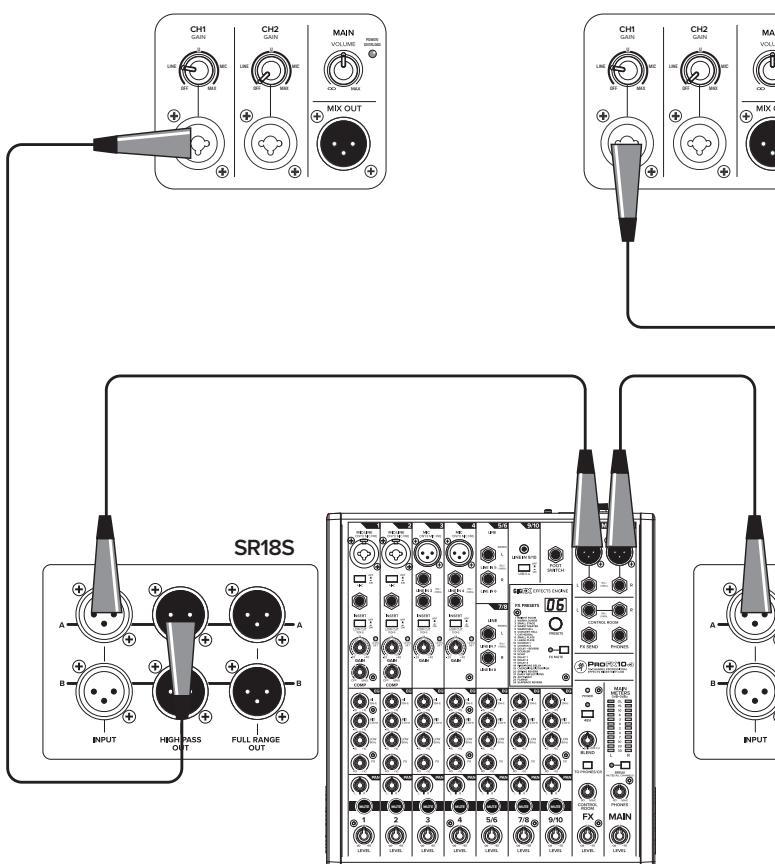
PA System with two powered subwoofers
