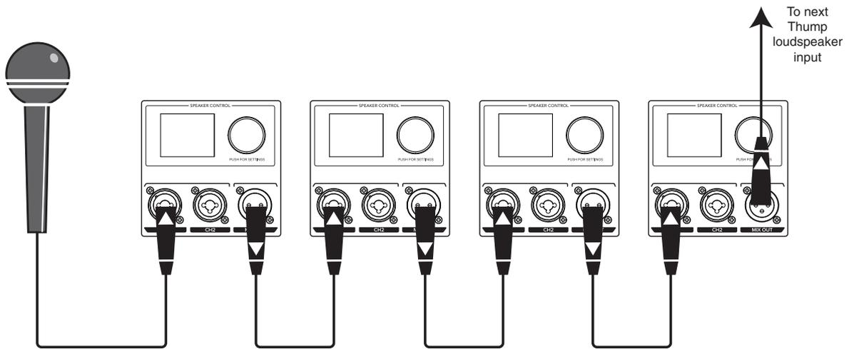
Thump loudspeakers may be daisy-chained via the male XLR connector labeled "MIX OUT". Simply plug the signal source (i.e., mixer output or microphone) into the input jack(s), and patch that loudspeaker's mix out jack to the next loudspeaker's input jack, and so on, daisy-chaining multiple Thump loudspeakers. See above for visual representations of daisy-chaining.
