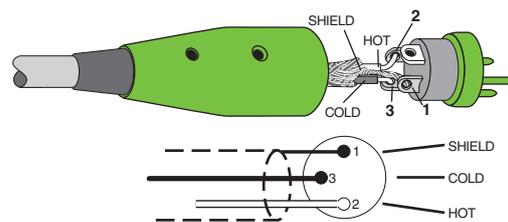
In addition to accepting a balanced mic signal using an XLR connector, these input channels may also accept 1/4" line-level signals driven by balanced or unbalanced sources.
