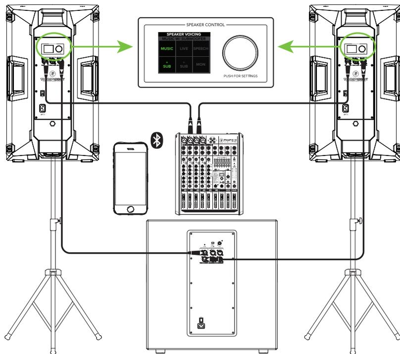
If you desire a little more boom, add a Thump18S subwoofer to the mix. Here, the L/R outputs of a ProFX8v2 mixer are connected directly to the CH1 inputs of each Thump12BST loudspeaker. Then the Mix Out of each loudspeaker is connected to the channel A and B inputs of a single Thump18S subwoofer. Don't forget to set the Speaker Modes to Music + Sub.
