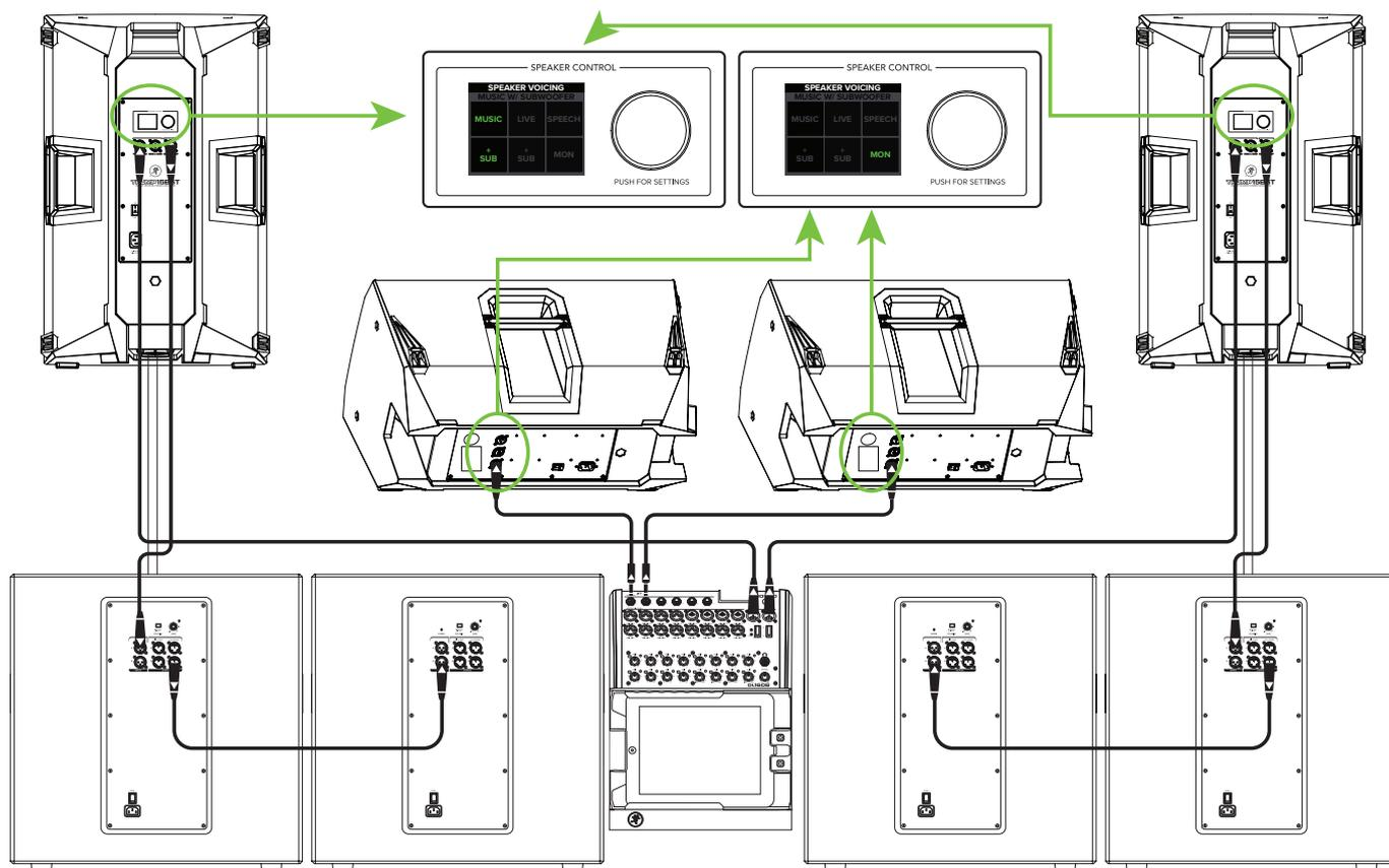
Here's how to set up a large club system. In this example, the L/R outputs of a DL1608 mixer are connected directly to the CH1 inputs of a pair of Thump15BST loudspeakers. The Speaker Modes of these PA loudspeakers may be set to Music + Sub.
