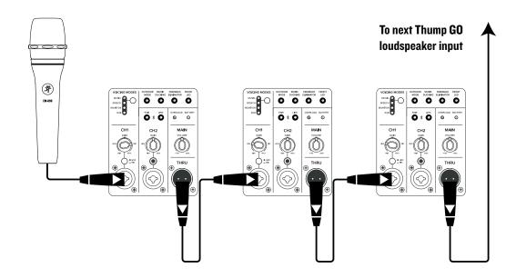
Thump GO loudspeakers may be daisy-chained via the male XLR connector labeled "THRU". Simply plug the signal source (i.e., mixer output or microphone) into the input jack(s), and patch that loudspeaker's thru jack to the next loudspeaker's input jack, and so on, daisy-chaining multiple Thump GO loudspeakers. See above for visual representations of daisy-chaining.
