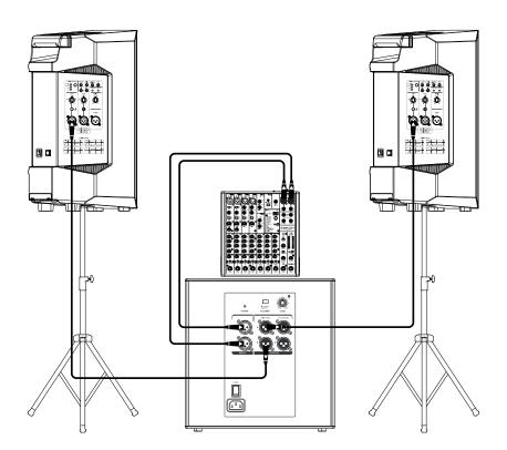
If you desire a little more boom, add a Thump 18S subwoofer to the mix. Here, the L/R outputs of a ProFX10v3 mixer are connected directly to the channel A and B inputs of the Thump 18S subwoofer. Then the High-Pass Outs of the subwoofer are connected to the channel 1 inputs of a pair of Thump GO loudspeakers. The gain knob on both should be set to Line. Here you will want to set the Voicing Mode to 'Music'.
