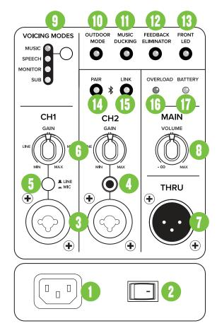
In addition to accepting a balanced mic signal using an XLR connector, these input channels may also accept 1/4" line-level signals driven by balanced or unbalanced sources.
