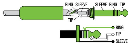
To connect unbalanced lines to these inputs, use a 1/4" mono (TS) phone plug, wired as follows:
