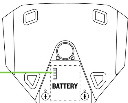
There are finger grips on each side of the battery, close to where the “battery” text is located. Remove the battery from captivity by lifting it straight up to freedom.
