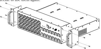
2. Using the Phillips screwdriver, attach the two new, recessed rack ears – one on each side – on the front side of the mixer using the same screws that were just removed.
