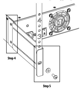
6. Using the Phillips screwdriver, attach each bracket adapter to the corresponding rear rack ear with the M4 Pan Phillips screws and locking washers, as shown below. Tighten the screws enough to securely engage the lock washers. In other words, tighten the screws only until the lock washers are seated flush to the metal.
