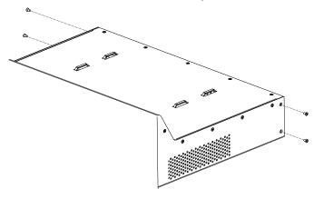
2. Using the hex key, attach the two bracket adapters – one on each side – on the rear side of the mixer through the fixed diameter holes using the M3 hex screws.
