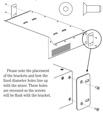
3. Place the mixer in the rack *at the intended location* and secure the front in place with four rack screws<sup>1</sup> (not supplied).
