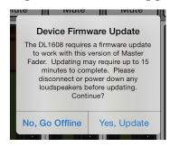
You will need to do a force update on the mixer when going back to a previous version of Master Fader (after using V4.6.1). **NOTE:** If using a Static IP address for your DL Series Mixer, an update may fail to begin properly. Similarly, a force update will fail in the same way. If either of these happen, you will need to temporarily configure the DL hardware to use Dynamic IP addressing.
